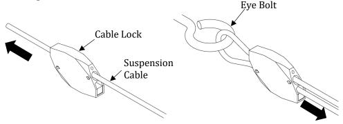
5. You can tighten the suspension cable using a catenary tensioning tool or loosen the cable using a cable release key on the cable lock.
